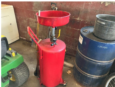
Oil Reclaiming Unit
